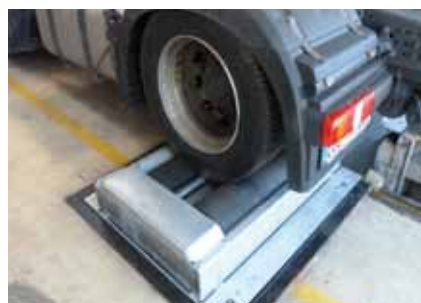
Last-Simulation, bis zu 200 mm Hub Load-Simulation, lifted up to 200 mm
