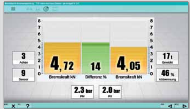
Graphical user interface can be customized: Scale displayable in clock or bar diagram style
